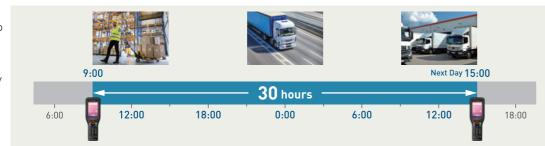
\*JEITA G mode: a bar code is read twice every 10 seconds with 1 KB of data being transmitted once, the wireless LAN is in power-saving mode, the backlight is on, and data is transferred via FTP. Actual battery life might vary depending on the operating environment and system settings.
